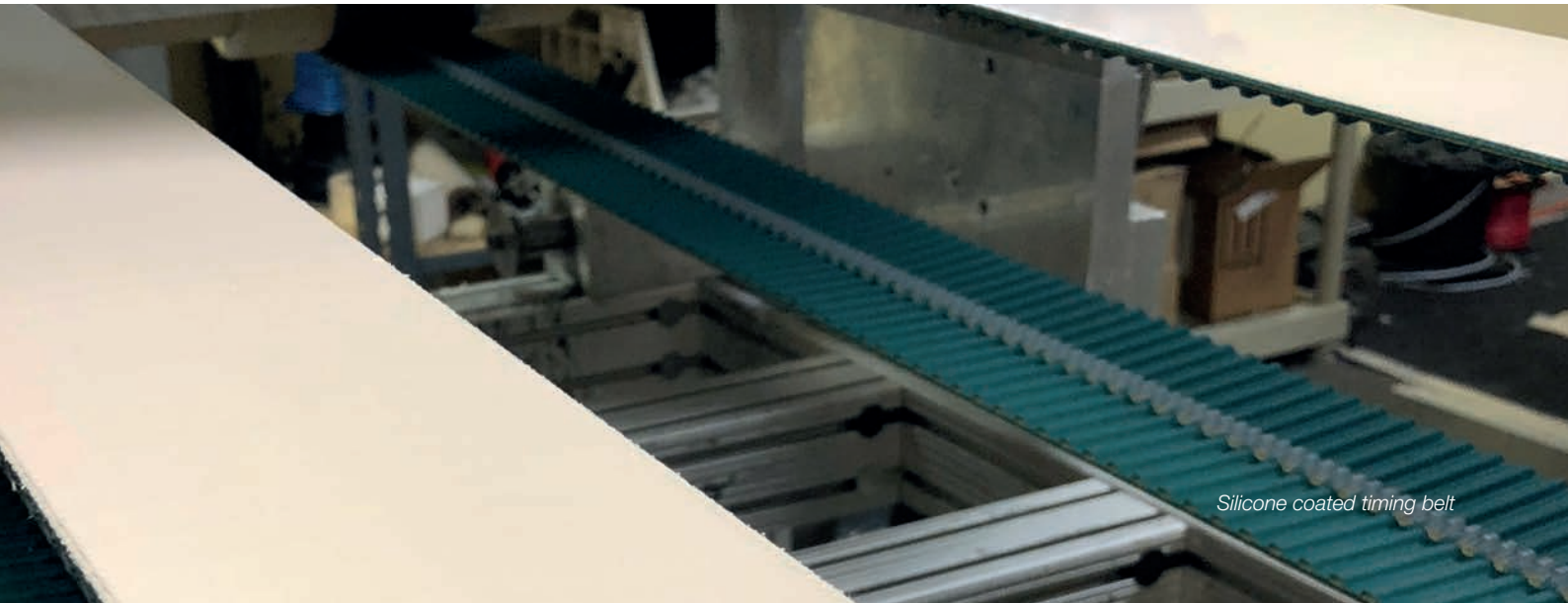
Silicone coated foam on Megapower substrate
