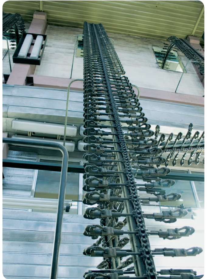
SKF Hollow Pin Chains used on a newspaper conveyor
